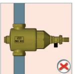
The dirt separator should be placed on the return line before the boiler, in such a way as to catch all the impurities that might damage the boiler and pumps. It is recommended that the dirt separator is installed between two isolating valves for maintenance.
