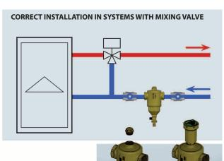
A FAR automatic air vent valve can be installed simply by removing the upper plug and screwing the valve onto the dirt separator.
